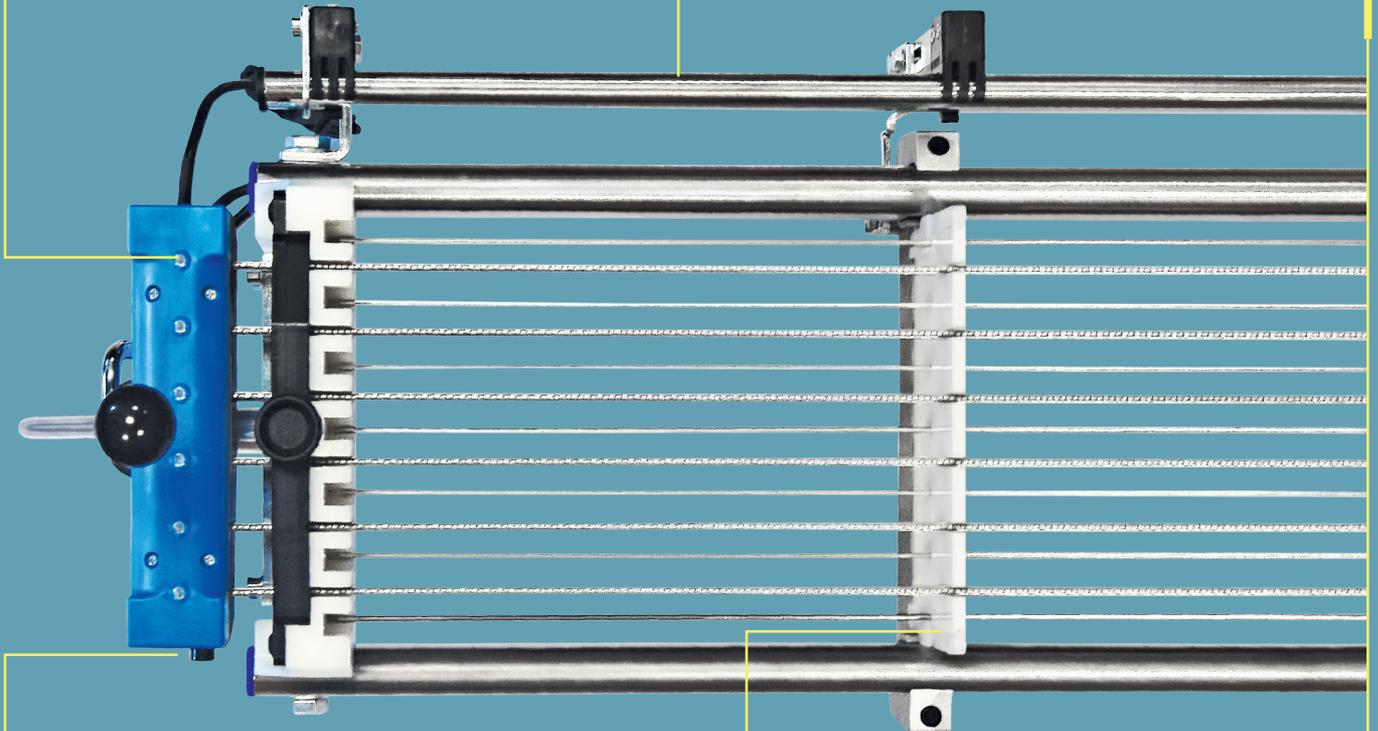
Optional device CFC able to indicate when the broken thread belongs to the waste selvage
