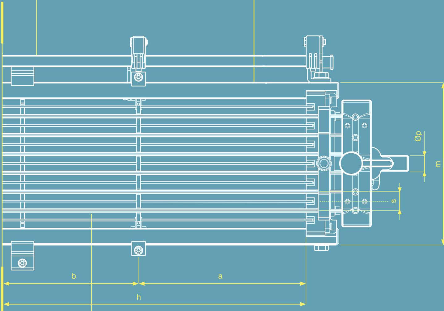
Contact bars made by antimagnetic stainless steel (material that prevents rust) insulated with polyester, the result of a tested construction technique
